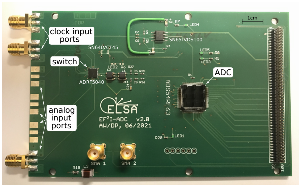
Figure 4.10: Photo of the second and final version of the Digitization board
