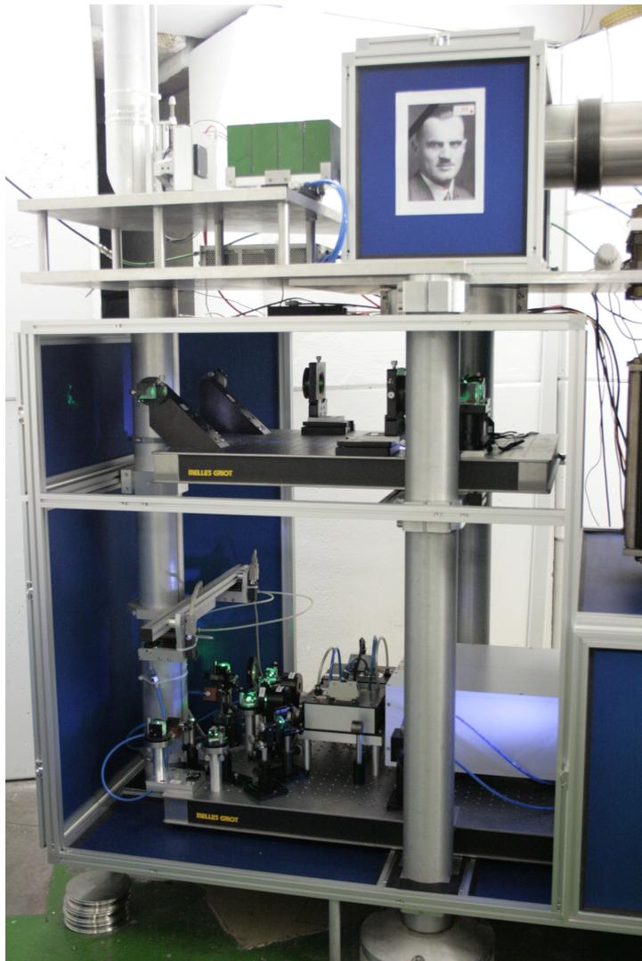
Figure 3.2: The optical table in its current state. The detector system is already in place on the rear end of the uppermost plate.
