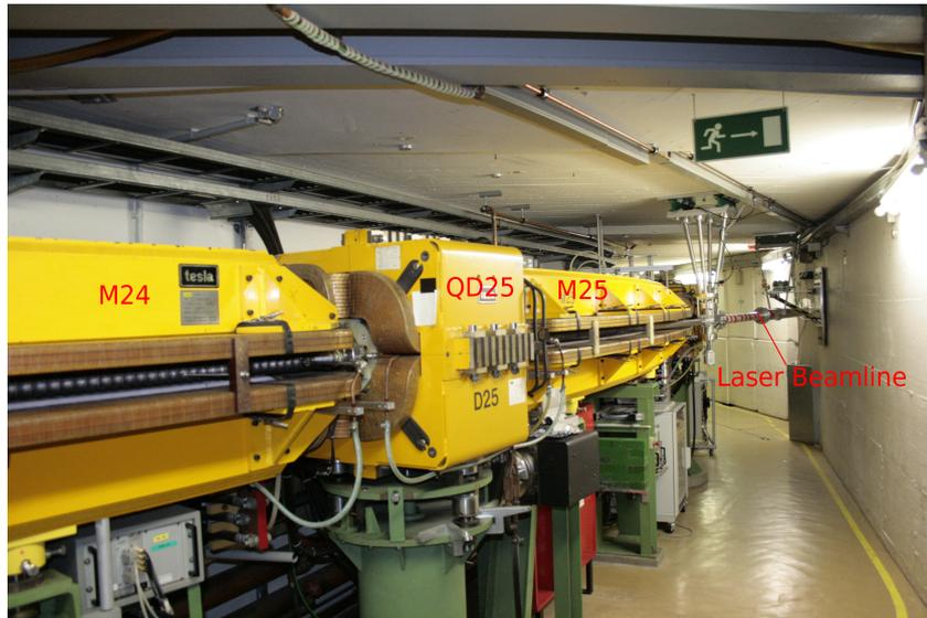
Figure 3.4: The Compton beamline in the ELSA tunnel. The optical beamline enters the electron beampipe in the M25 magnet and leaves the stretcher ring in the M24 magnet.
